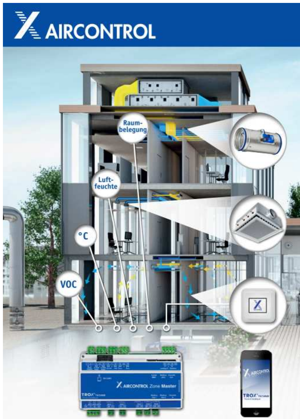
Picture: Efficient room control with X-AIRCONTROL. The integration of the X-CUBE air handling unit, volume flow controllers, heating and cooling components, and air-water systems into an overall system offers huge economic and ecological benefits.
